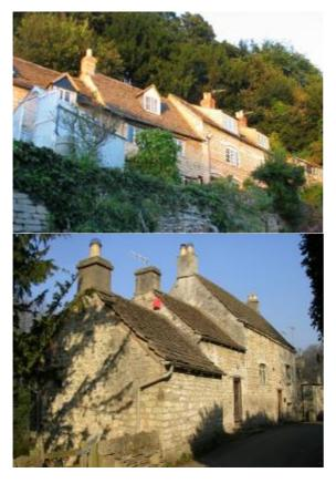
These terraces of cottages demonstrate buildings added on to each other, probably at different periods. Note how the roof heights are staggered to cope with the hillside.
